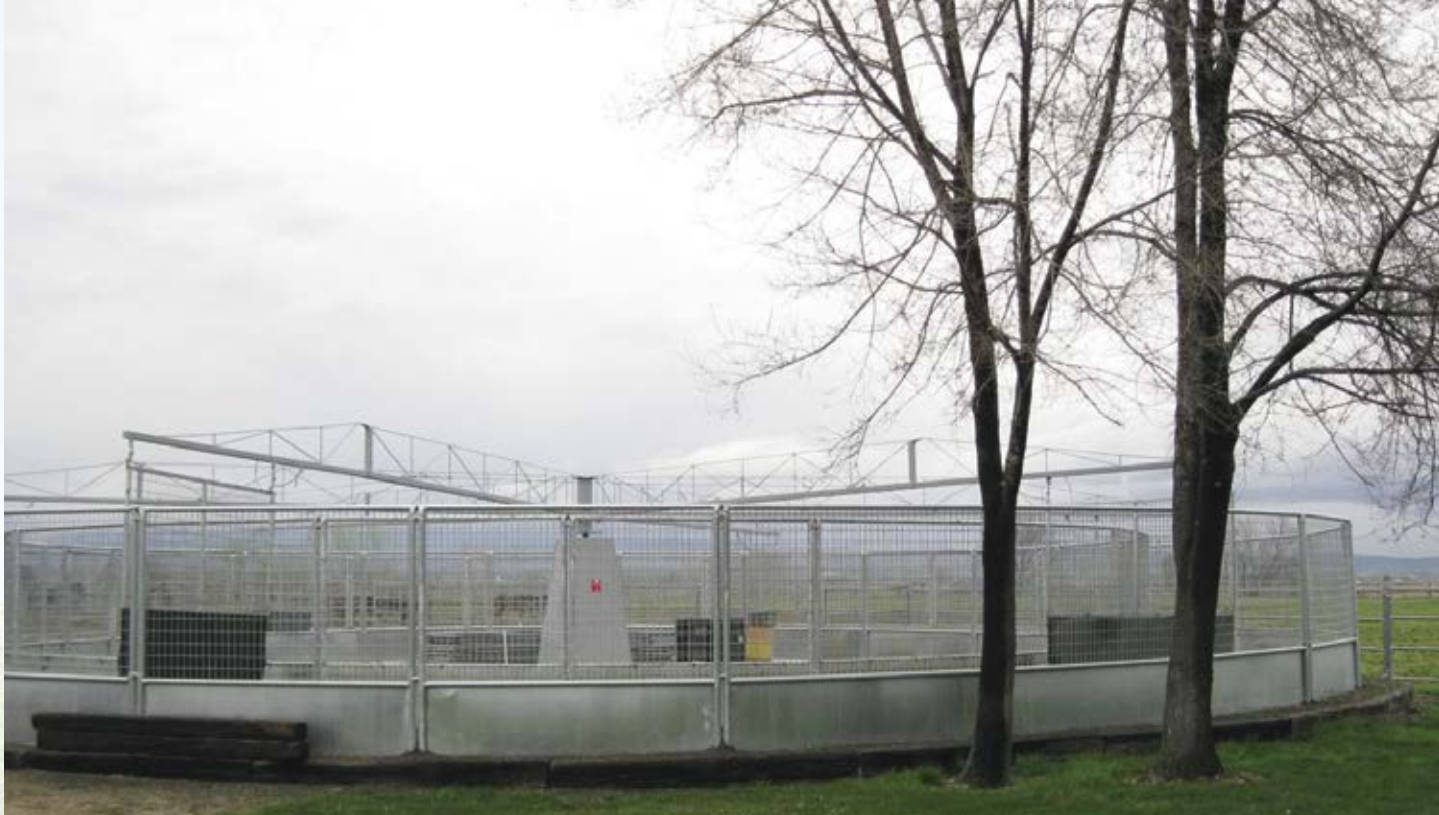
The Eurocizer machine allows horses to be untethered as they move freely throughout an exercise session.
